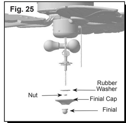
26. Feed pull chain through the center hole in the glass globe, rubber washer and nut. Lift the glass globe and rubber washer over the threaded rod.
