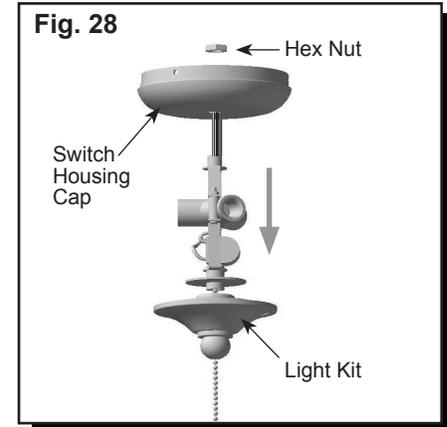
29. Align the notch in the switch housing cap with the reverse switch. Then lift the switch housing cap into the switch housing and re-insert the three screws and washers that were previously removed. Use a Phillips screwdriver (not included) to secure all screws. Plug the hole in the switch housing cap with the plastic cap (Fig.29).
