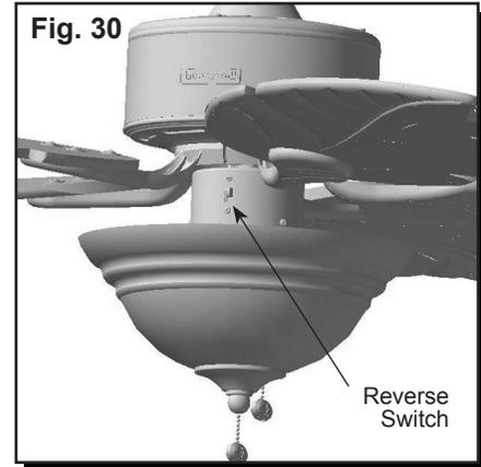
31. **In warmer weather**, push the reverse switch down, which will result in downward airflow creating a wind chill effect (Fig. 31).
